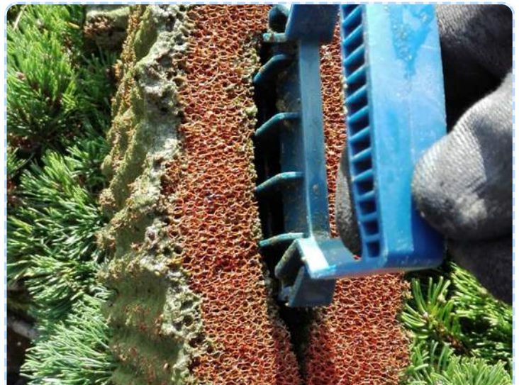
Algae flocculated and captured on filter
