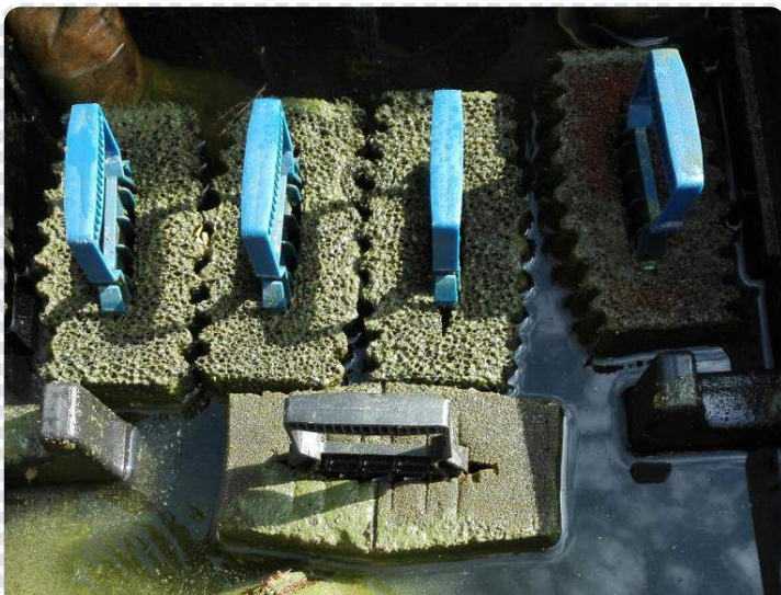
Filter units clogged with algae
