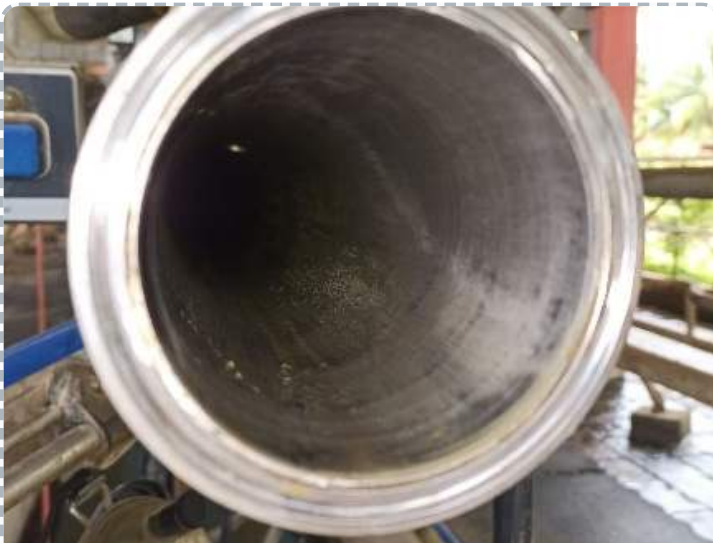
Pipe interior with milk scale buildup
