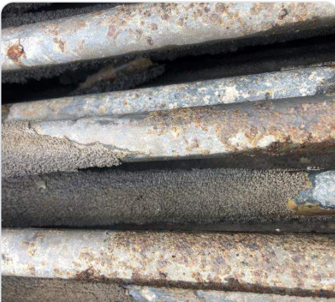
Condenser 3 tubes with heavy scale
