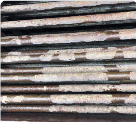
Condenser 3 tubes with heavy scale
