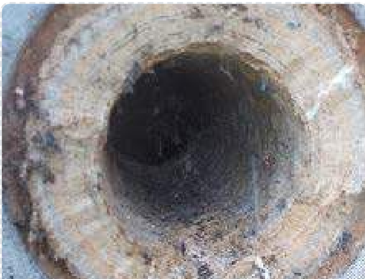
Heavy struvite scale in centrate pipe
