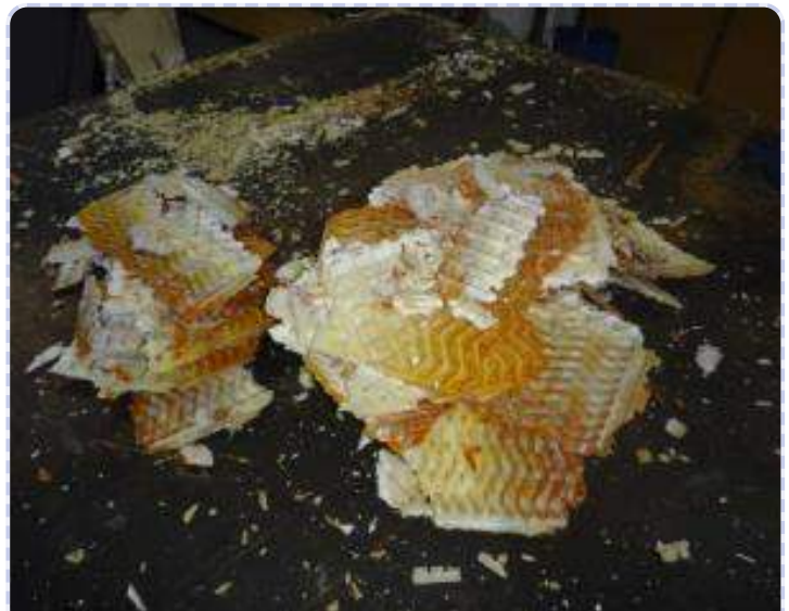
Scale removed from FWG plates
