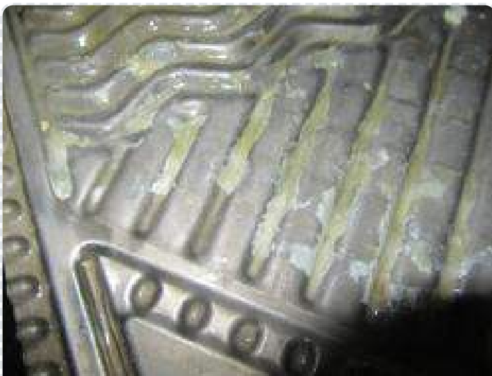
FWG plates with heavy scale build-up
