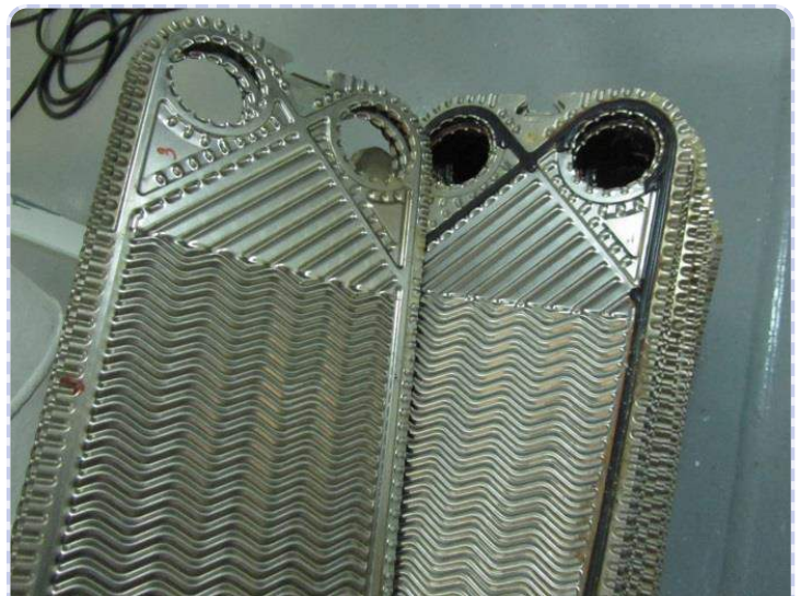
FWG plates clean with loose scale only
