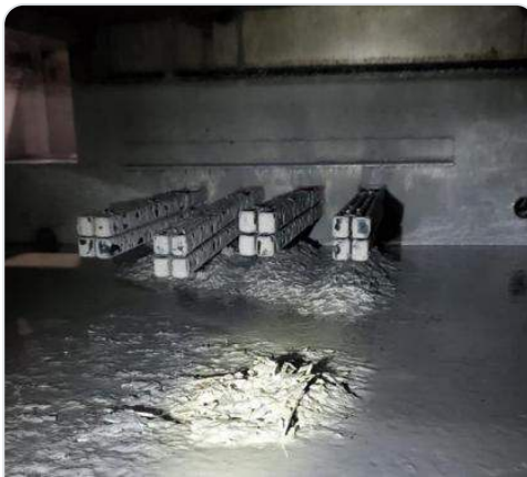
Scale deposits inside washer system before treatment
