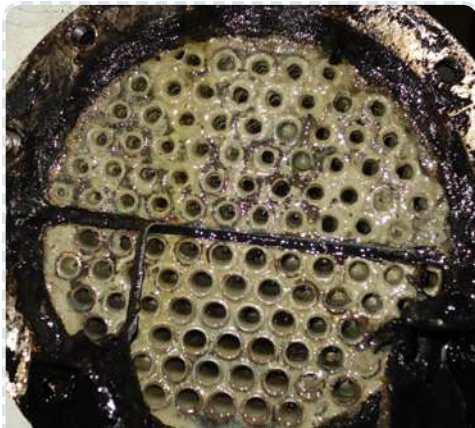
Heat exchanger plate fouled with scale
