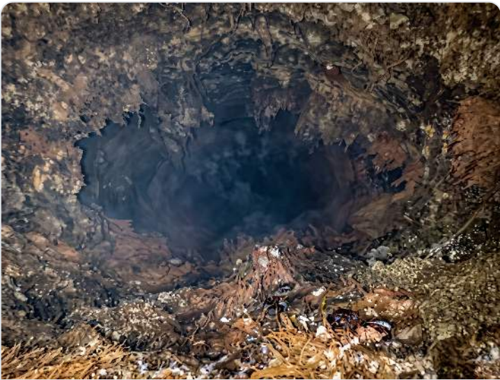
Control line with mussel fouling
