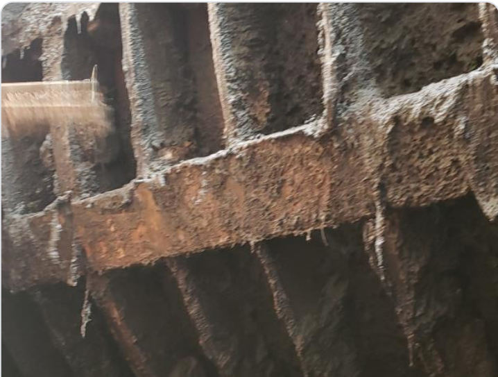
Hard struvite inside the screw press
