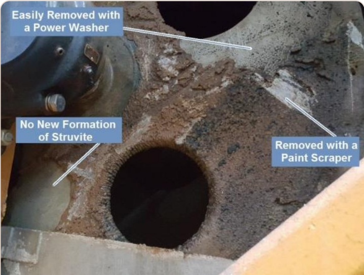
Drum surface after the 90-day trial
